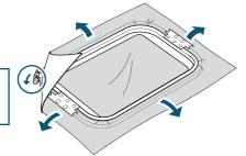
5. Tighten the adjustment screw on the outer frame.
