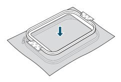
4. Loosely tighten the adjustment screw on the outer frame, and then smooth out the cloth within the frame to remove any looseness or wrinkles.
