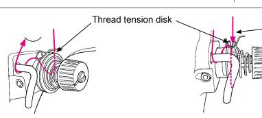
Pass the thread through the clearance between the two thread tension disks.
