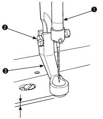
Minimum clearance between the throat plate and the presser foot: 0.5 mm (at the time of shipment)
