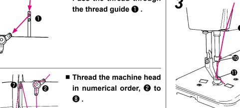
■ Pass the thread through the thread guides 9 and **O**.
