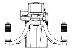
When you press the "start button" on the right handlebar, the sewing machine will start sewing according to your settings. When you press the "start button" again, the sewing machine will stop sewing.
