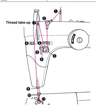
\* Bring the thread take-up **1** to the upper end of its stroke. Then, pass the thread through it.
